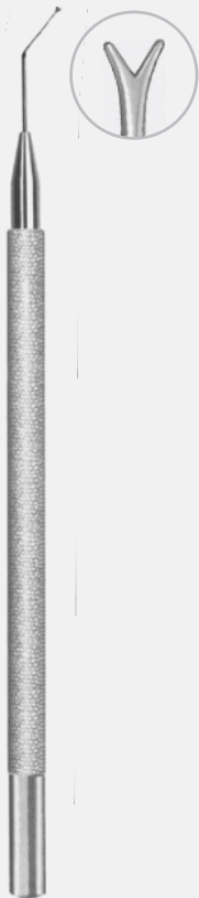
OP-689-01 Bechert Nucleus Rotator 0.78 mm Horizontally Forked Tip With Angled to Tip Length of 7 mm Overall Length 11.5 cm (4 1/2")
