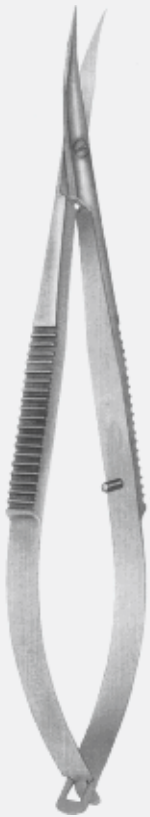
SS-683-11 Westcott Stitch Scissor Curved, Very Sharp Pointed Tips 20 mm Long Blades With Max. 10 mm Cutting Edge Overall Length 11.5 cm (4 ½")
